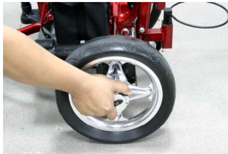
Depress the quick release catch, whilst putting wheel in position on the axle
